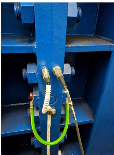
Accelerometer placed on the stator joint in radial direction
