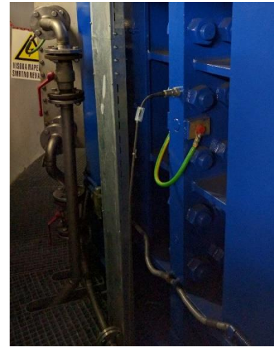
Accelerometer placed on the stator joint in radial direction
