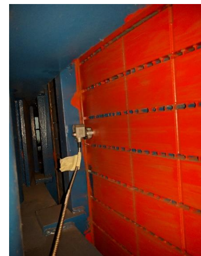
Velocity meter placed on the stator core, at the right side of the stator joint, in the middle of the core (up-down)
