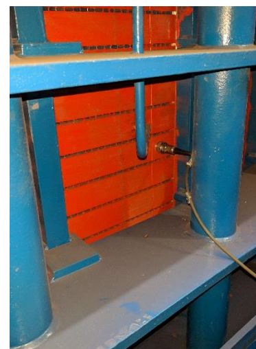
Accelerometer placed on the stator core, in the middle of the, temporarily removed, cooling unit
